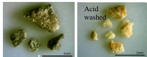
Figure 10: Particles before and after acid washing.
